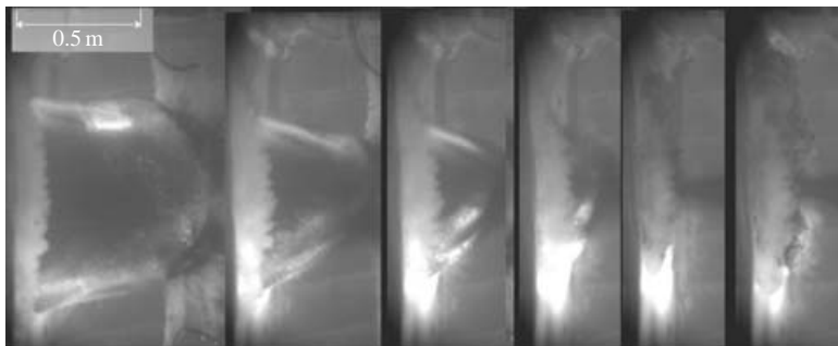
FIGURE 15. As for figure 13, experimental bubble shapes at t = 82 , 91, 94, 97, 100 and t = 104 ms.
